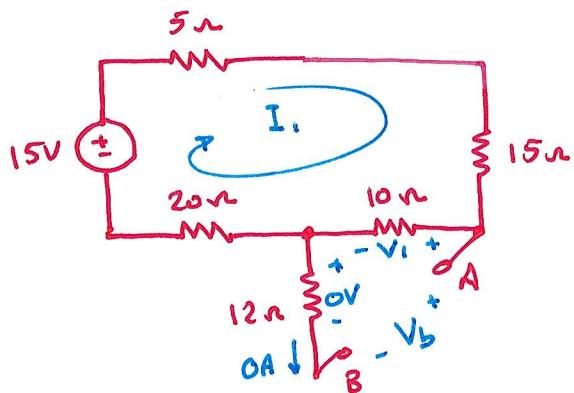
$$I_1 = \frac{15V}{5\Omega + 15\Omega + 10\Omega + 20\Omega}$$
