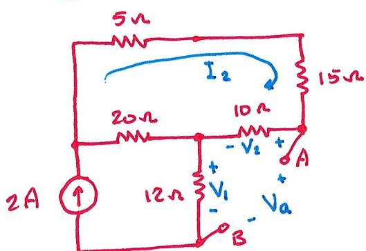
$$V_1 = (12\Omega)(2A) = 24V$$
