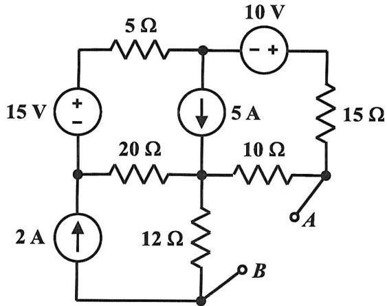
Find the Thévenin equivalent circuit with respect to terminals *A* and *B*.
